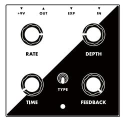
**FEEDBACK** - This control brings focus and resonance to the sweep of a sound. At minimum position, sweeps are smooth and neutral. At medium position, sweeps begin to peak musically. At maximum position, the sound of a sweep becomes rigid and metallic.
