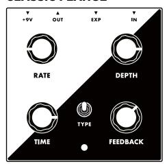
**TIME** - At maximum position you can craft traditional or vocal, metallic flange sounds. As the Time control position is reduced, delay time is increased and sounds become thicker and warmer. At minimum position, the MF FLANGE is capable of approaching analog chorus style sounds.
