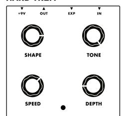
**TONE -** This control affects the Tremolo signal only leaving the dry signal untouched. At maximum, all frequencies are affected by the tremolo. As the Tone control position is decreased, the effect of the tremolo becomes more subtle. From the mid position down, the Tone control can be used to dial in sounds that impact only low frequencies in your guitar or to shape classic rotary swirl and phase-like effects.
