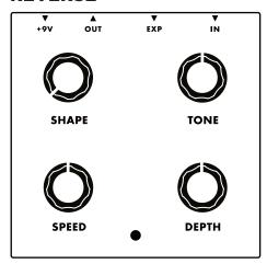
**DEPTH -** At minimum the tremolo effect is subtle and mostly dry. As Depth is increased more tremolo effect is blended in the mix causing phase cancellation and addition effects. At center position the sound will begin to gallop and swing. This impact on the sound varies significantly depending on Speed. At maximum position, the tremolo speed doubles and all sound is sent through the Tone control.
