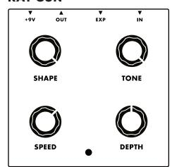
SHAPE - Sweeps between modulation waveshapes. Center position has a smooth rise and fall. This is great for creating optical tremolo sounds. Hard right has a hard impact followed by a smooth decline. This creates abrupt and percussive behavior that is very musical when paired with the Tone knob. Hard left has a smooth lift and abrupt drop off which creates a sound similar to a reverse effect at slower speeds and a rotary speaker at higher speeds.
