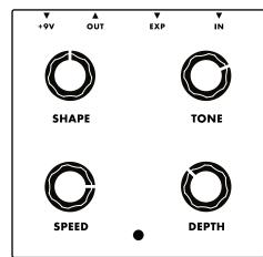
**SPEED -** Sets the overall Tremolo rate. At slower settings the sound is swirling, lush, and transformative. As the Speed is increased the sound becomes tighter and more like a rotary speaker. The Shape and Depth controls will directly affect the perceived speed and rhythm of your Tremolo as they are increased from minimum to maximum position.
