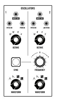
This is where the sound of the synthesizer is born. Grandmother provides two oscillators of almost identical design, each with its own Octave and Waveform settings. Oscillator 2 is equipped with a **FREQUENCY** knob to detune it from Oscillator 1.
