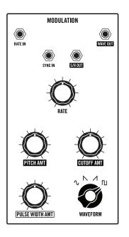
Modulation is an important aspect of programming and playing synthesizers. In short, whenever one signal is used to change the value of another – it is known as modulation. Grandmother has a dedicated Modulation section that can apply modulation to multiple destinations at once, and in varying amounts. This Modulation section is based around an analog oscillator that operates in the low-frequency range, and is commonly known as an LFO (Low Frequency Oscillator).
