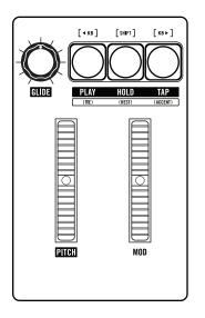
Grandmother's Left-Hand Controller is home to numerous performance and programming controls including **PITCH** and **MOD** wheels, a **GLIDE** control, and transport controls for the Arpeggiator and Sequencer.
