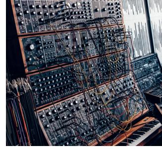
The Moog 35 is connected to Hannes' DAW via a Moon Modular MIDI-to-CV and MIDI-to-clock interface, which goes into the Moon 568 pattern gate sequencer that controls the Moog 35 and the DFAM.
